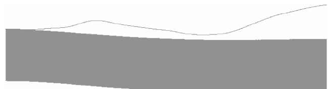
Fig. 21 Deformed shape: G_{Ic} = 1.27 N/mm, current increment = 2800; total increment = 7000.
