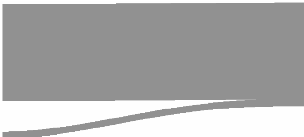
Fig. 15 Deformed configuration for the case with end-shortening of 1 mm at t = 0.08 s.
