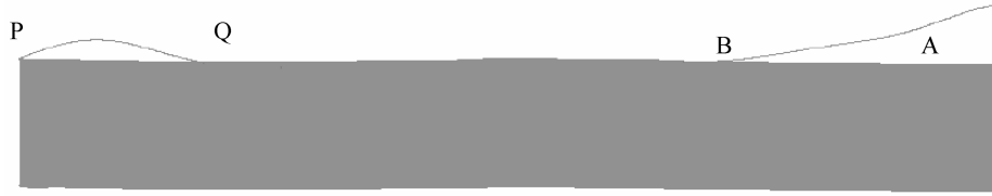
Fig. 19 Case 2: dynamic delamination deformed shape for the case with G_{Ic} = 1.27 N/mm, t = 0.016 s; total inc = 7000.
